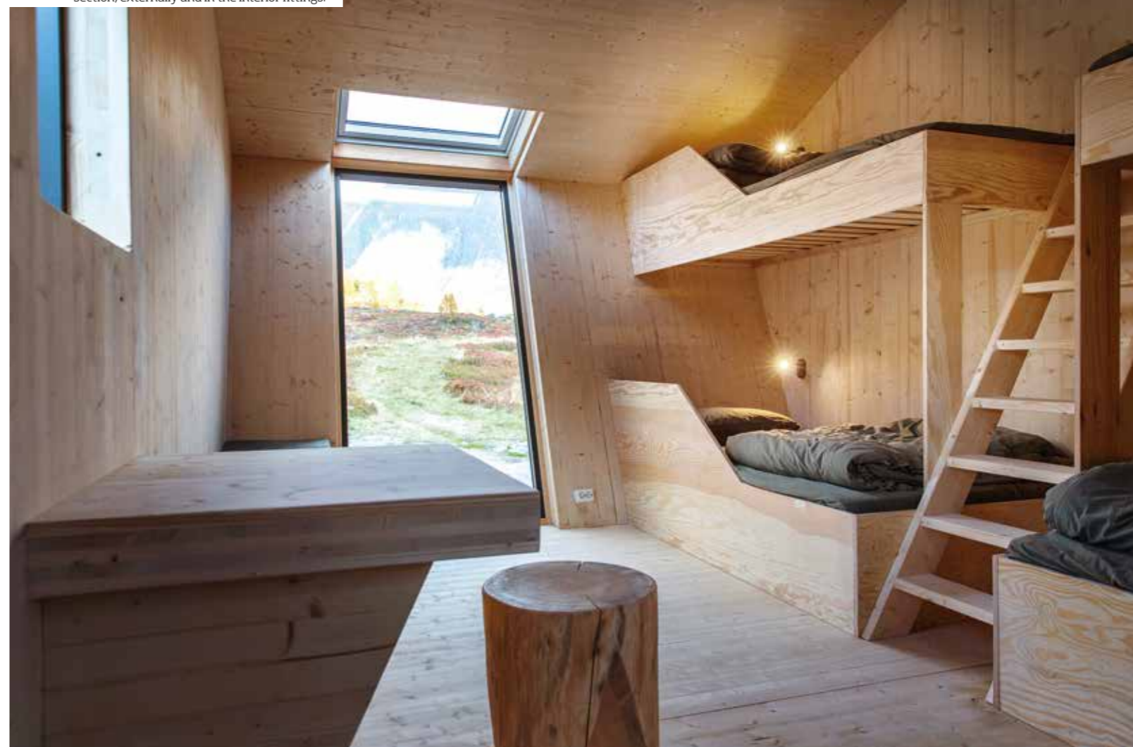
The playful shape of the cabins helps to slow the strong winds that sweep in from the valley. All the cabins embrace the five-sided cross-section, externally and in the interior fittings.
